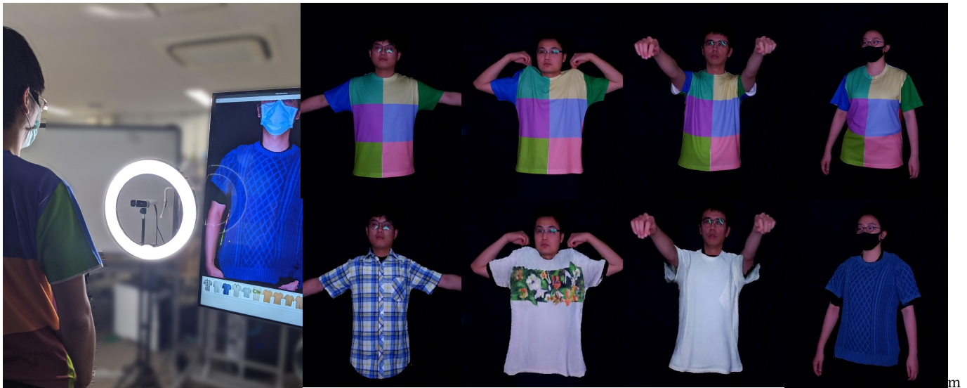
Figure 1: Our real-time system allows the user to virtually try-on various garments using different interactions, such as stretching the body and pulling the garment. The user first wears the color-coded measurement garment (top row), and our system synthesizes the target garments with detailed wrinkles according to different motions.
