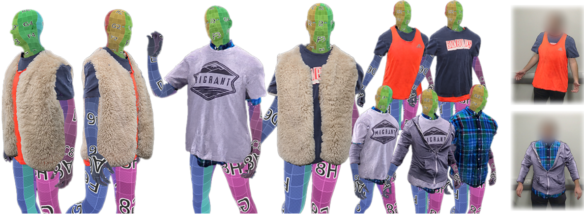
Figure 1: We present a novel method for interactive mix-and-match avatar dressing of multilayer Gaussian garments. To address penetrations between the body and the garment, as well as between the garment layers, we incorporate a novel screenspace visibility culling method inside the 3D Gaussian splatting renderer. We also show a webcam-based interactive virtual try-on.
