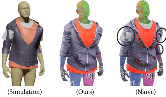
Figure 7: Even when simulation results in large penetrations (left), we are often still able to recover high-quality visual results (center). A naïve approach results in large penetrations, in addition to other artifacts (right).
