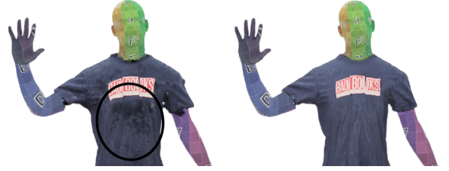
Figure 12: We compare Gaussians optimized with our second optimization (right) and with only our first optimization (left). By including our second optimization pass, we both ensure Gaussians are well aligned to the mesh surface, and form a full opacity cover of the mesh. In the circled section, Gaussians fail to form a full cover—the black background used in our visualizer is visible through the Gaussians.
