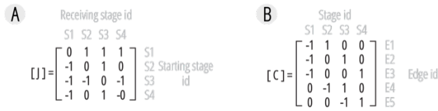
Figure 24: The graphical representation of the interconnected compliant mechanism shown in Figure 3C-E. The rigid stages and compliant joints' connectivity are represented by a (A) directed adjacency matrix [J] and an (B) incidence matrix [C], respectively. The entries in the matrix indicate the direction of connection – 0: not connected; -1: sender of connection; 1: receiver of connection.
